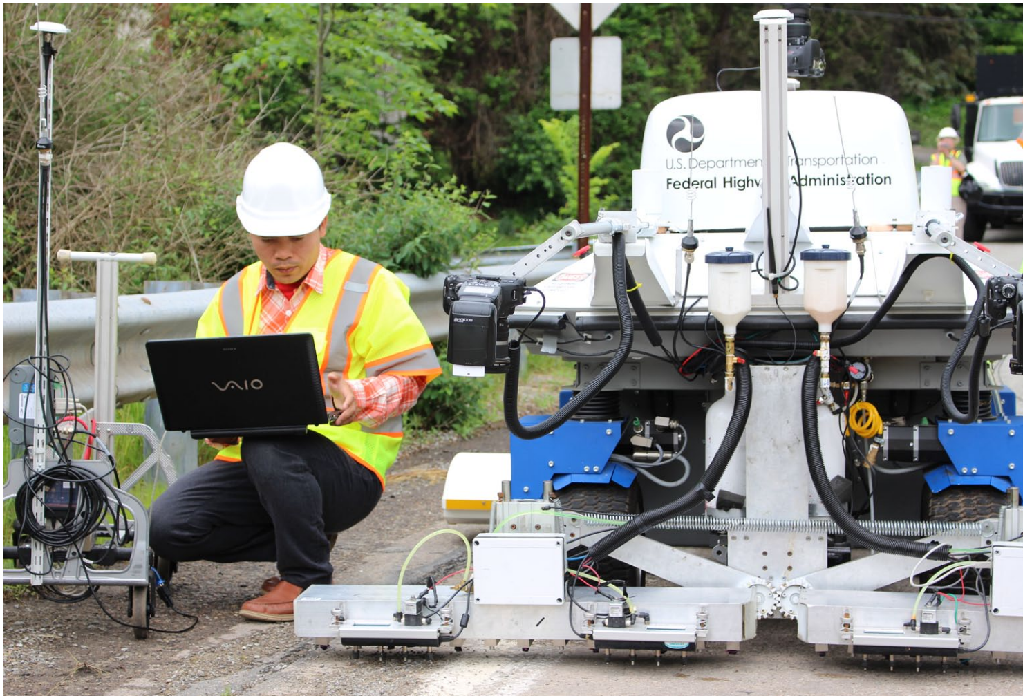
RABIT™ bridge deck assessment tool inspecting road surface
